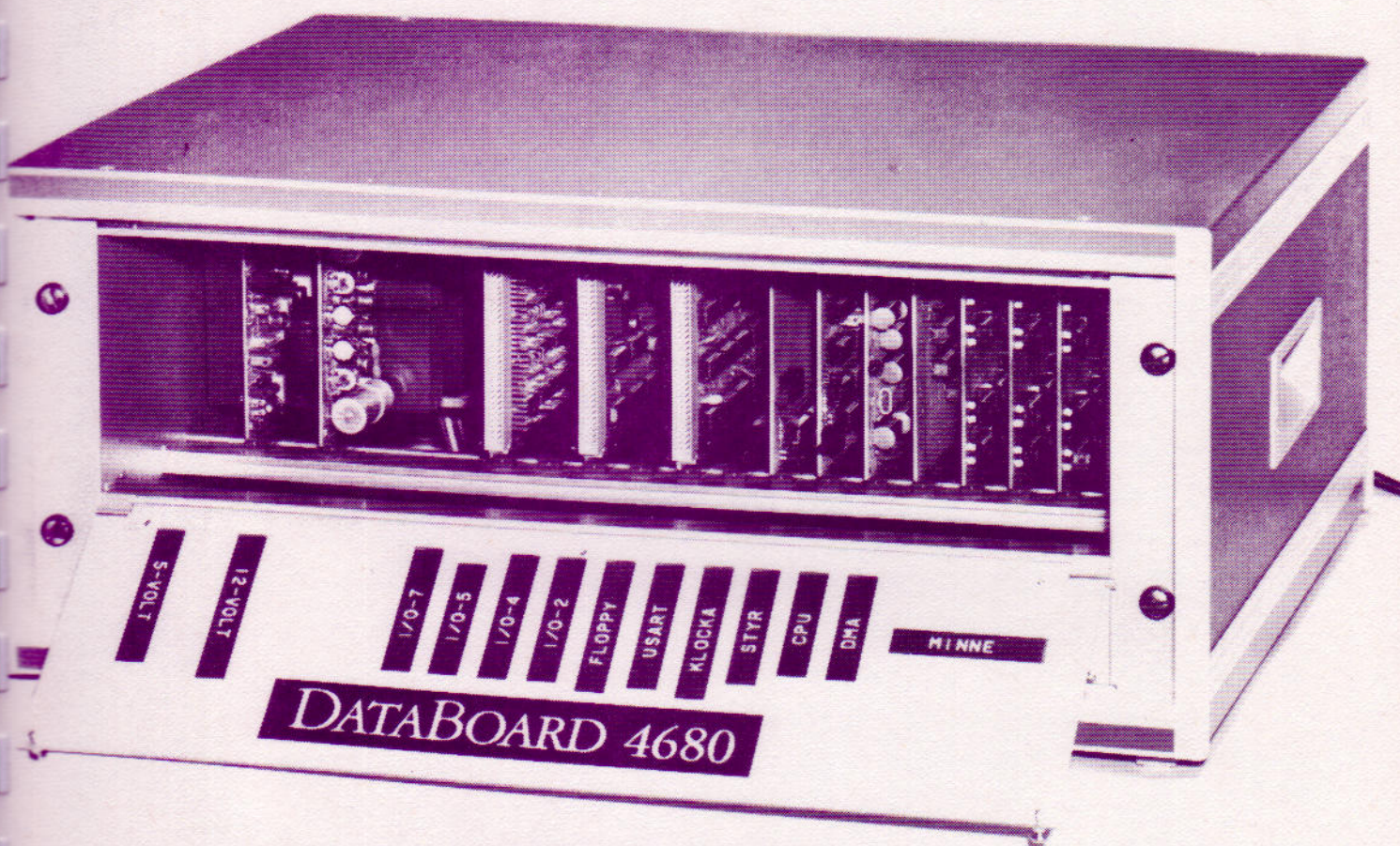
Pic.2 System built-up in a 19" rack.
