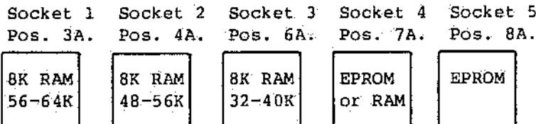
The jumpers S4 select the addressing range for the sockets 5 and 4 (Pos. 8A and 7A). The address bit A13 limits the range in socket 4 when an 8K RAM chip is used.
