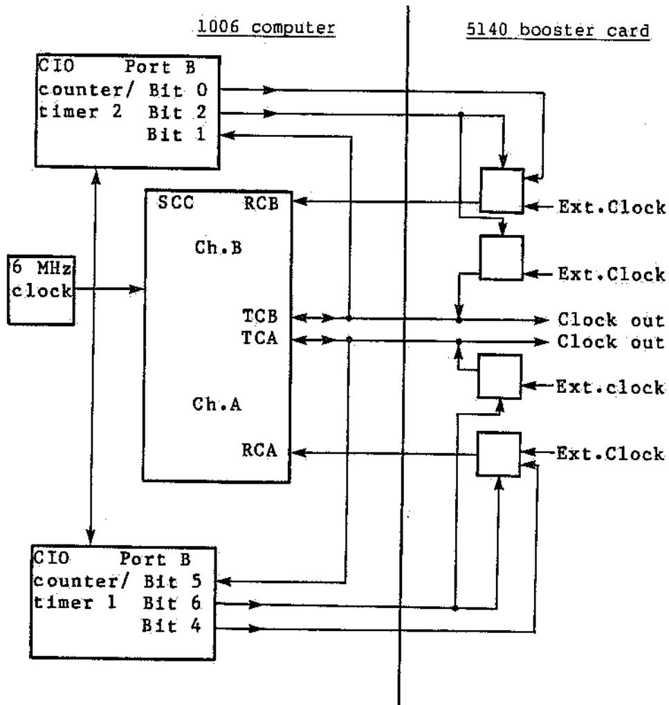
Baudrates (transmit and receive clocks) can be generated from:
