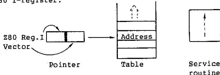
In the service routine, before returning from the interrupt, the interrupt source must be reset by resetting the "IUS-bit" in the CIO or the SCC. Resetting this bit is through commands to the CIO or SCC and is done instead of the RETI instruction, used on previous Zilog products. The RETI does not work on the SCC or the CIO. See reference (2) and (3).
