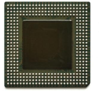
Pin Grid Array (PGA) Package
